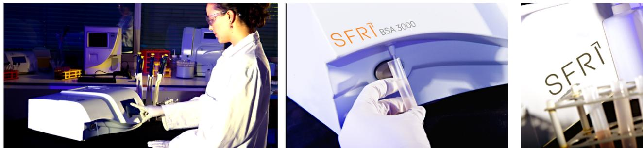
The BSA 3000 is a semi-automated biochemistry instrument used to perform routine clinical chemistry tests. The BSA 3000 performs certain operations automatically such as heating, analyzing, calculating and printing; the reaction solutions being prepared manually by the operator beforehand.
